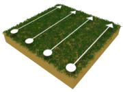
Return to the previous starting point and take a step to the left (without scanning): This is the starting point of the next scan line.
