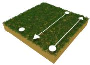
Remain at the end of the scan line and take a step to the left (without scanning).
