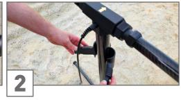
Open the sensor clamp, position the Super Sensor at the correct height (arrow pointing in scan direction), and close the clamp again.
