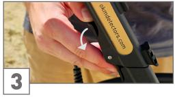
Use the locking levers to loosen the single segments of the Telescopic Rod.
