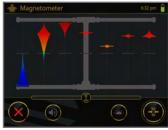
The graph shows **BLUE** peaks if the probe is pointing at the negative magnetic pole of a ferrous object.
