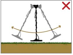
Do not sweep the coil along the ground. Avoid too large distances to the ground – especially at the sides.
