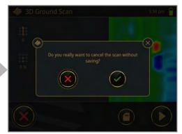
Confirm with  $\checkmark$  to discard the scan and return to the Main Menu OR return to your scan procedure with  $\checkmark$ .
