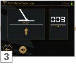
When finished, both arrows are in the target position and the 'quietest' ground value is displayed on the right. This value is saved for the current measurement.
