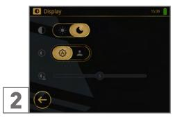
Select Automatic Brightness to allow the screen Select Manual Brightness and move the slider to adjust automatically to the ambient light.
