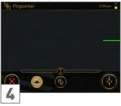
Tap on to perform a Ground Balance. The graphs will be reset to the zero line.
