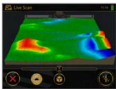
A combination of a **BLUE** and a **RED** spot most likely indicates the magnetic poles of a ferro-magnetic object.
