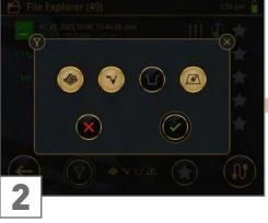
Tap on the operating modes to show/hide the corresponding scan files. Confirm with  $\checkmark$ .
