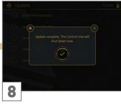
Confirm with  $\checkmark$  to shut down the Control Unit. After restarting it, you can use the detector as usual.
