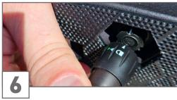
Plug the probe into the Control Unit - see 3.4 Backstrap + Control Unit on page 15.
