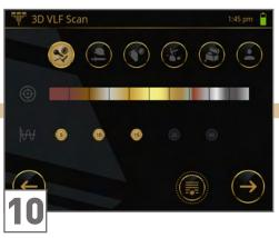
Select Recovery Mode: Level 5 is preset as default for 3D VLF Scan to provide the best depth performance. Tap repeatedly to toggle between 5 levels to adjust the Recovery Time according to your needs.
