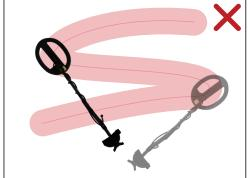
Make sure that the scanned areas overlap with each swing to ensure that the scan field is scanned without skipping potential targets.
