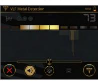
The detected object results in a signal within the grayed-out Target-ID zones.
