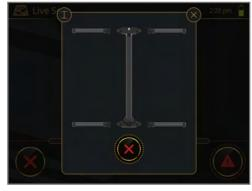
If you see this screen, the SuperSense System is not connected properly. Check the Probe connection and/or the Extenders – see 3.2 SuperSense System on page 13.
