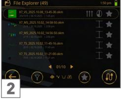
Open File Explorer. The digit(s) in brackets indicates the total number of saved scan files. and push the Knob to open a scan file.
