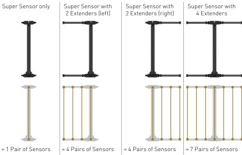
If you attach 2 Extenders, they must both be plugged in at the bottom and top on the same side (right OR left). The pairs of sensors must be complete in order to work properly.
