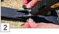
Insert the coil mount of the Telescopic Rod into the shaft adapter of the VLF Coil. Fix it with the mounting screw and tighten it so that the coil does not move.
