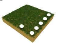
Return to your first starting point without scanning and take one step to the left: This is the starting point of the second scan line.
