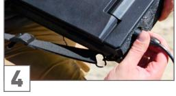
Lift the Control Unit to see the socket at the rear, and plug in the probe.
