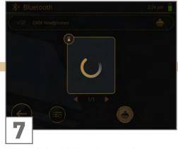
Wait until the pairing and connecting process is complete. The LEDs above Knob flashes blue while pairing and connecting:
