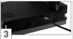
Plug the opposite end of the charging cable into the Control Unit to start charging.
