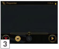
Hold the Super Sensor above neutral ground, and start with  $\triangleright$ .
