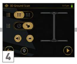
For rough terrain, you can select the Impulse Mode Manual : Every single impulse (scan value) requires the Knob/ to be pressed.
