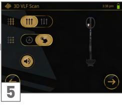
Regardless of the selected scan mode and impulse mode, you can tap on **1** to switch ON / OFF the Sound.
