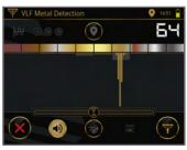
Strong signal detected in one of the active Target-ID zones. Displayed Target-ID is 64.
