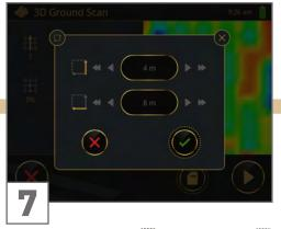
Enter the Field Length \_\_\_\_ and Field Width \_\_\_\_ that you actually measured: Tap on the arrows (left/right) or turn the Knob.
