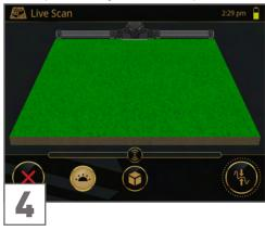
Tap on 🔥 to perform a Ground Balance. The visualization will be reset to green surface.
