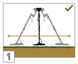
Swing the coil from one side to the other, closely and parallel to the ground (approx. 5 cm | 2" above the soil surface).
