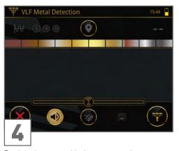
During the ground balance procedure, the detector reselects the 'quietest' signal channel and returns to the scan screen. The sensitivity will be reset to zero.
