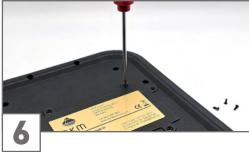
Close the battery compartment. Lock its cover with the 6 Torx T10 screws.
