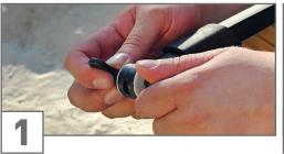
Unscrew the mounting screw from the coil mount at the Telescopic Rod. Make sure the rubber washers are seated next to the shaft before attaching the VLF Coil.
