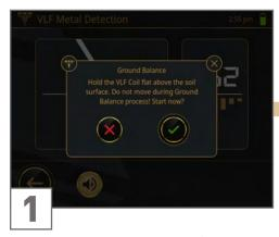
Place the coil on neutral ground (no objects underground). Hold it approx. 5 cm | 2" above the soil surface and do not move it. As soon as you are ready, start the Ground Balance with ...
