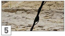
Wrap the cable tightly around the Telescopic Rod to avoid false signals while detecting.
