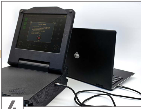
4 (1) Connect the Control Unit with the Windows notebook via USB-C cable.
