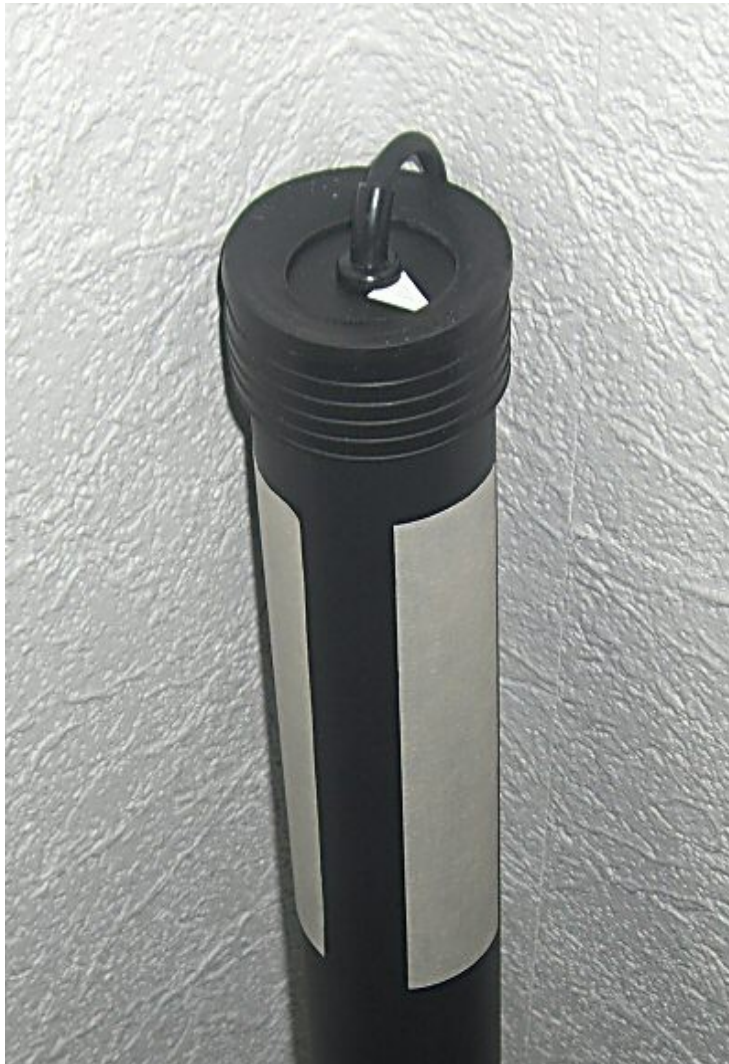
Illustration 9.2: Add additional marks to the Super Sensor aids in the scan.
