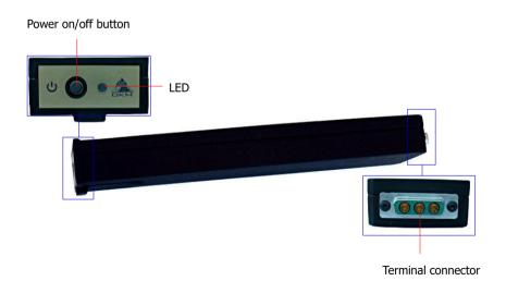
To turn on the Power Pack, the power on/off button should be pressed until the LED is shining. If the Power Pack cannot be powered on, it might be discharged to much and recharging is required (see section 6).
