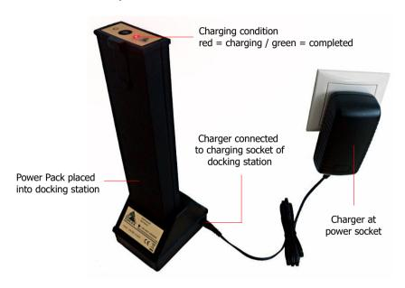
During the charging process of the Power Pack, the LED is blinking in red color. As soon as the LED blinks green, the Power Pack is charged completely and must be removed from the docking station. By that the Power Pack will turn off automatically.
