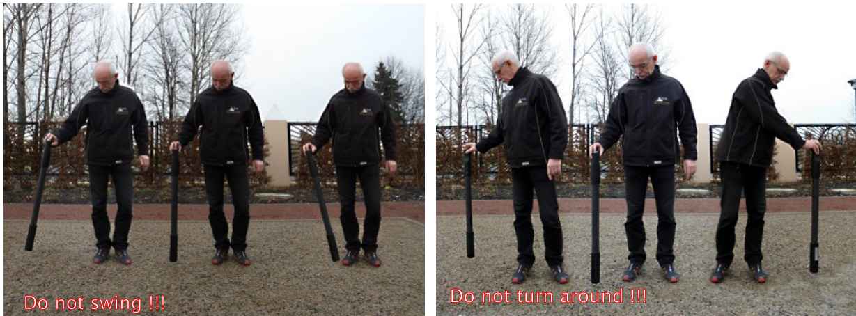
Figure 7.9: Pivoting or turning of the probe falsifies the measurement
