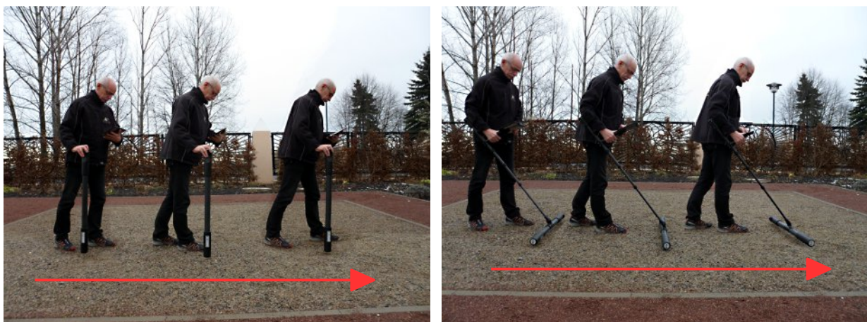
Figure 7.5: Ground Scan in vertical and horizontal mode
