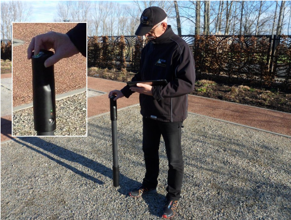
Figure 6.1: Using the detector in vertical mode
