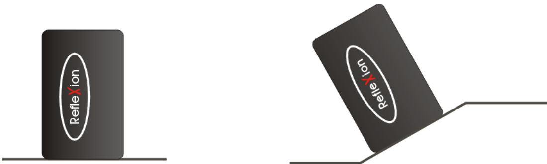
Figure 37: Right positioning of transmitter
