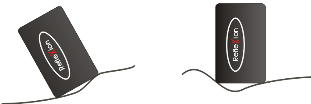
Figure 38: Wrong positioning of transmitter
