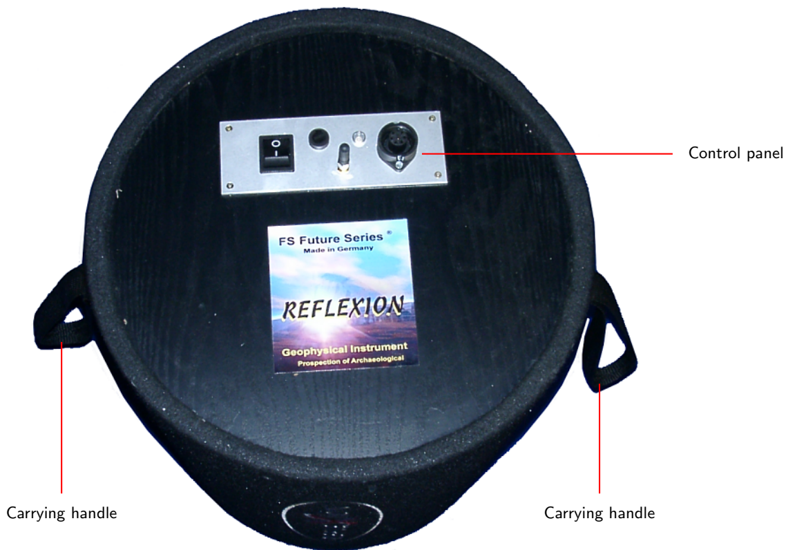
Figure 5: Transmitter with its components
