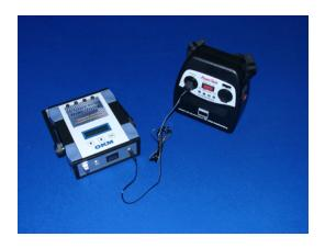
Figure 3: Connection of External Power Supply
