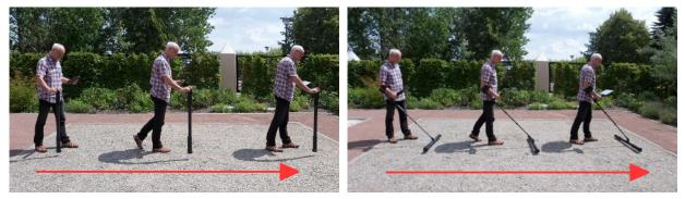
Figure 6.5: Ground Scan in vertical and horizontal mode
